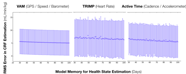
Figure 7: Comparison of sensor prediction performance based on changing the memory in the model in determining health state. Based on a p-value of 0.05, there were no statistically significant differences in choosing the memory value. Thus, we chose the established standard of 42 days for our model [21].
